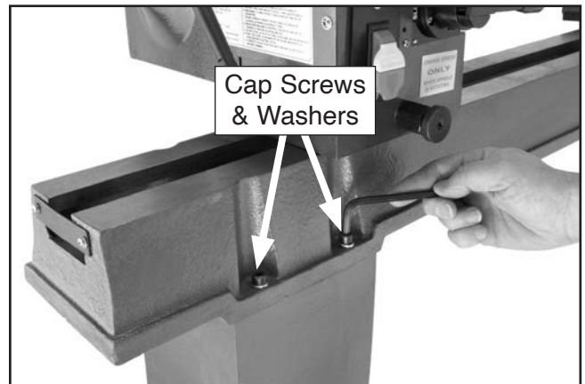
Figure 4. Example of securing lathe bed to stand legs.
