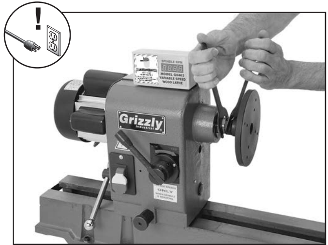
Figure 25. Tightening the faceplate onto the spindle.
