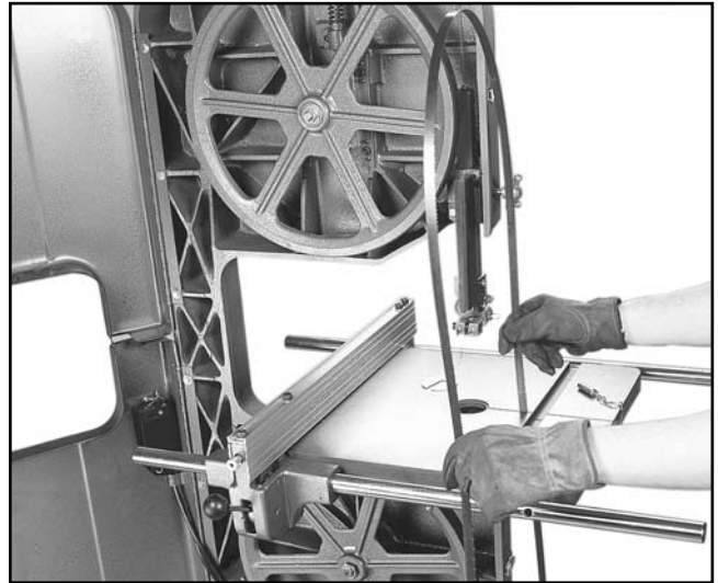
Figure 23. Changing blade with leather gloves.
