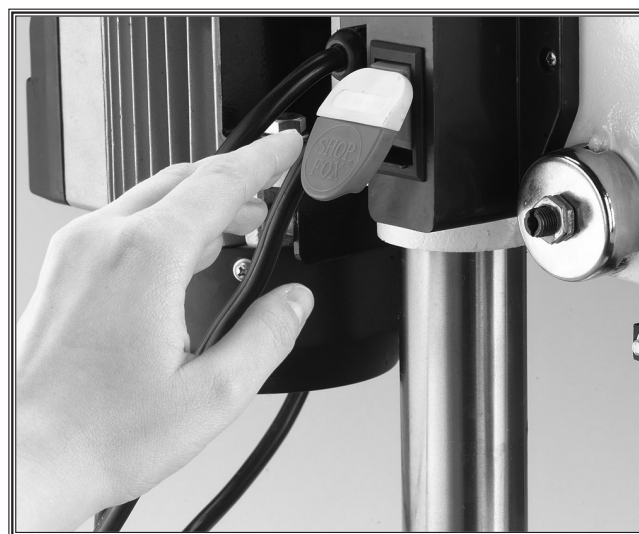
Figure 39. Hand poised over a typical stop switch.
