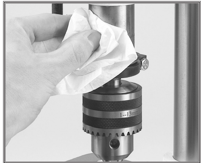
Figure 28. Clean and oil quill shaft.
