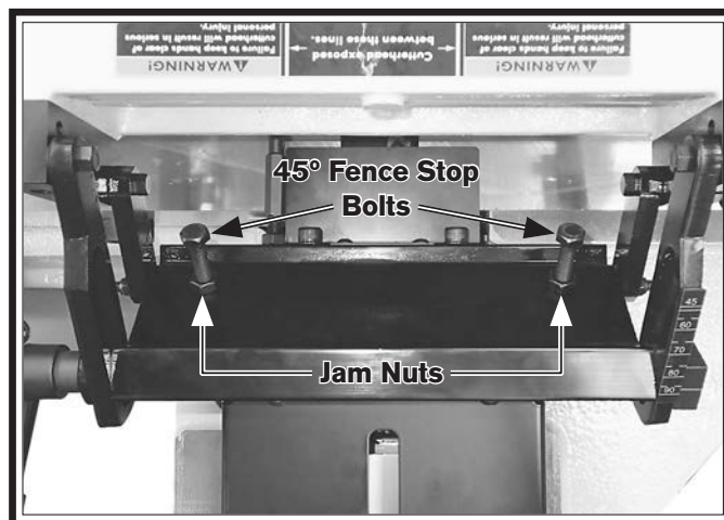
Figure 59. 45° outward fence stop components.
