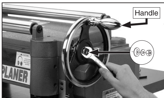
Figure 14. Installing handwheel on shaft.
