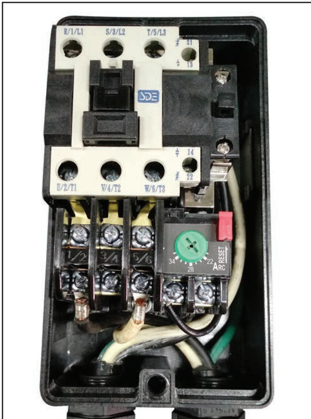
Figure 74. G1033Z magnetic switch with cover removed.
