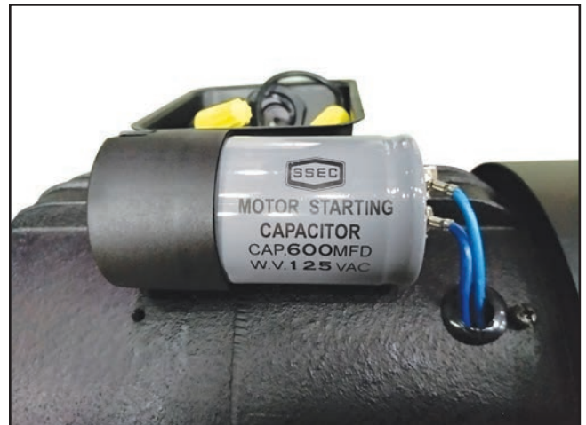
Figure 69. G1033 start capacitor.
