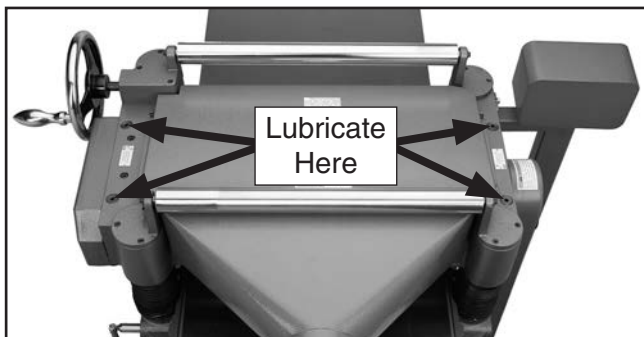
Figure 40. Lubrication locations for feed roller bushings.
