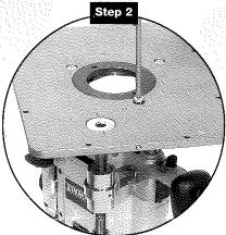
**Step 2** Position PlungeLift as shown over router base. (Do not remove brown sub-base.) Install and tighten (3) screws (supplied).
