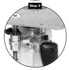
**Step 3** Orient support arm so that it is above attachement point on router. With support arm barely brushing against attachment point, install bolt, lock washer and both flat washers as shown. Tighten with 1/2" wrench.
