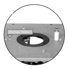
**Step 4** With the plunge lock lever in the unlocked position, rotate the crank handle clockwise to test for free motion. More resistance in the clockwise direction is normal due to the plunge springs in your router (do not remove the springs). If to much resistance is experienced;
