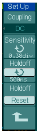
Figure 2- 63 Table 2- 39 The Trigger Set Up Menu (Settings for trigger coupling, trigger sensitivity and holdoff)
